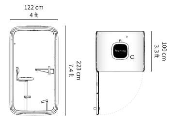
The door handedness can be changed on-demand with simple tools, by flipping the front frame in its place.
