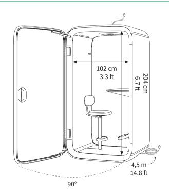
Power cord can be led out of the bottom corner of the pod or from the roof. The cord length outside the pods is 4,5 m / 14.8 ft
